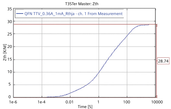
Figure 3: Z_{th} thermal impedance of a QFN package
