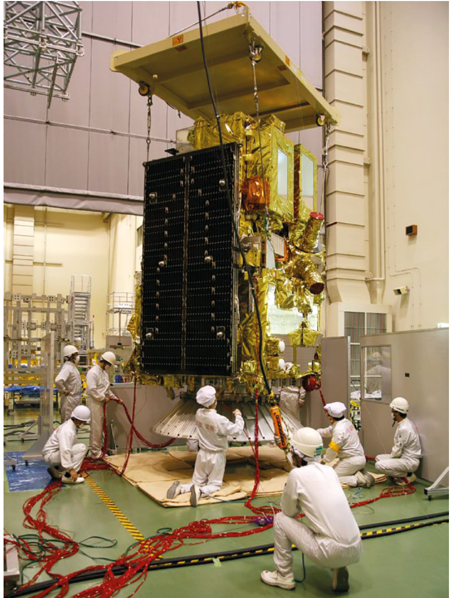
Figure 1: Instrumentation of satellite for vibration test: The Data Acquisition solution of Simcenter Testlab and SCADAS is engineered to acquire and process online data coming from hundreds of different sensors during vibe, pyro and acoustic tests.
