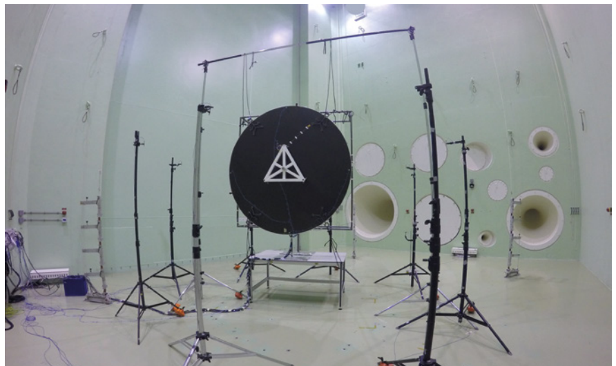
Figure 4: Simcenter Testlab Acoustic Control is the solution for closed loop control in reverberant chambers.
