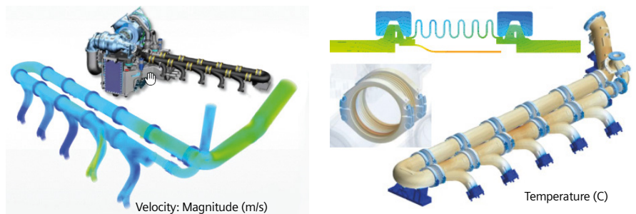
Figure 4: Fully embedded loose fluid/solid coupling approach for thermal analysis of e.g. the exhaust manifold
