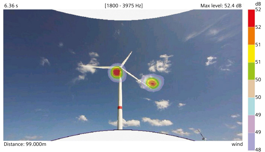
Figure 2: Simcenter Sound Camera - sound sources at nacelle and blade tip.
