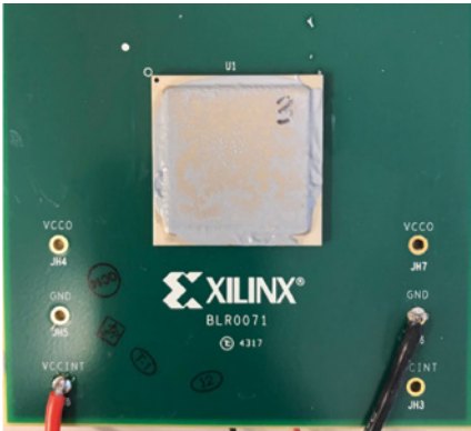
Figure 1: Xilinx Package mounted on JEDEC 2S2P PCB
