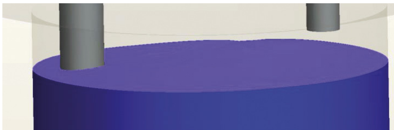
Figure 7. The air-water interface in the sump, showing a low level of deformation, indicating no vortex formation or air entrainment
