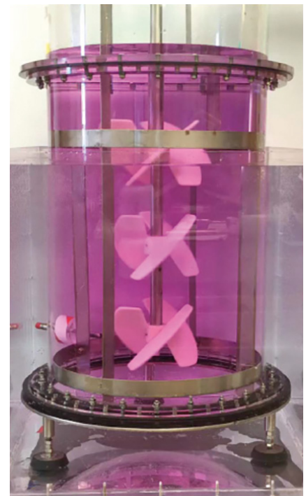
Figure 1: Experimental setups used for small-scale model testing of impeller configurations
