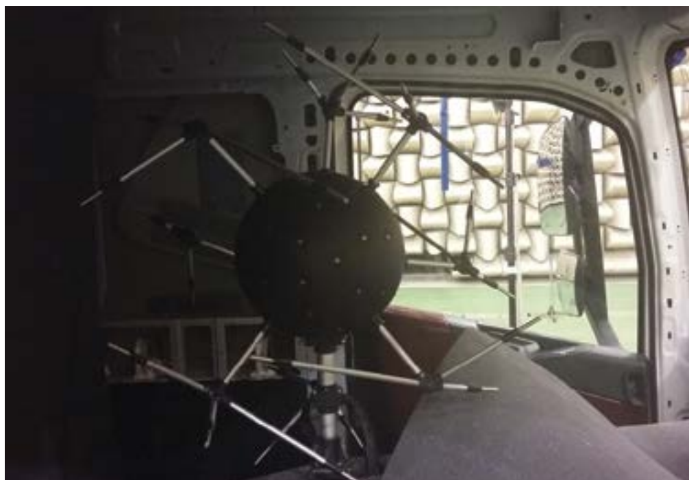
Figure 1: Spherical acoustic camera used to scan the inside of a truck's cabin
