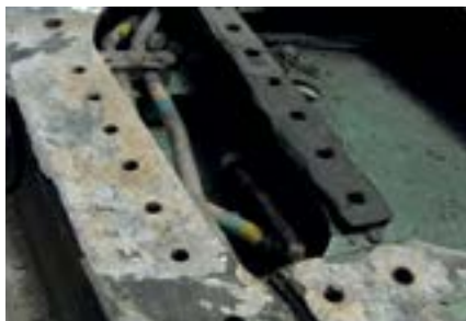
Figure 1: F-18 wing and airframe corrosion
