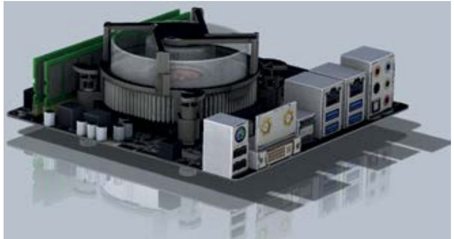
Figure 5: Board with egg replaced with stock CPU cooler
