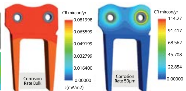
Figure 5: Corrosion rate on uncoated lug/bushing in an F-18 aircraft
