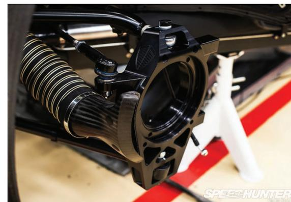
Figure 3. Brake cooling duct mounted on a Koenigsegg Agera upright (the baseline design). Klingelhofer, 2013, Ref 3.
