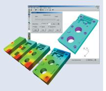
The MCAD geometry file is converted to an ACIS solid on import into FloMCAD Bridge. A desired simplification level is set on a slider bar, appropriate for the level of detail required. The model is then simplified, converted into FloTHERM objects and transferred to FloTHERM in a single operation.
