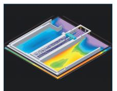
Chassis geometry pre-processed by FloMCAD Bridge and analyzed in FloTHERM
