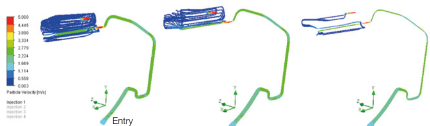
Figure 3. Virtual Debris test, Debris size from left to right (a) 0.2 mm (b) 0.3 mm (c) 0.5 mm
