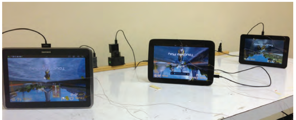
Figure 7. Images of three Different Tablets Running Riptide GP while Temperatures are being Monitored with Thermocouples.
