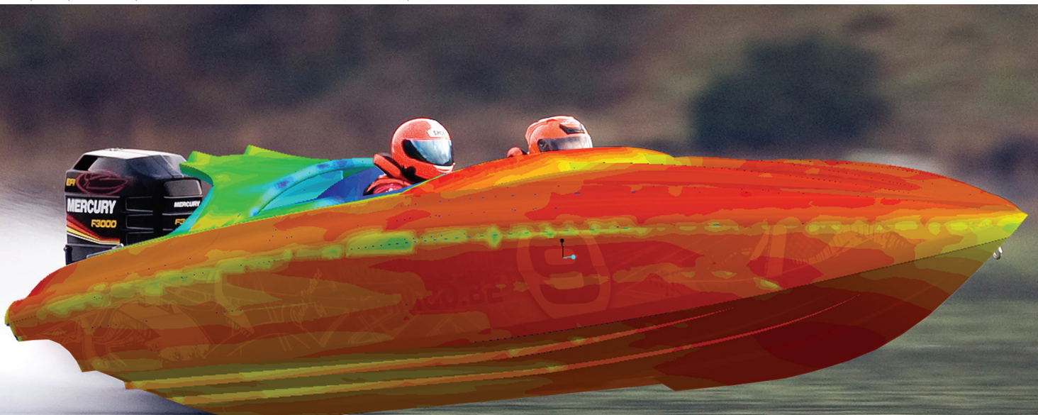
Figure 4. Record Breaking F2 Bernico Boat on Coniston Water in November 2009 with superimposed hull pressure contours from FloEFD simulation prediction
