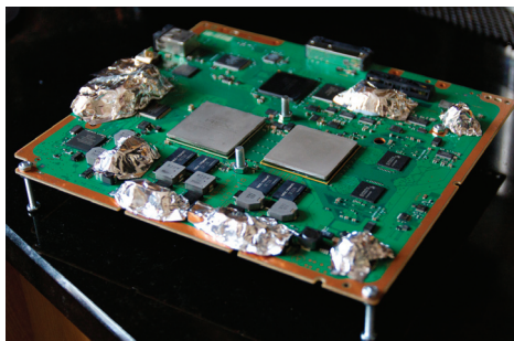
Figure 4. Bluetack and Foil Shielding Small Fast to Heat-up Components
