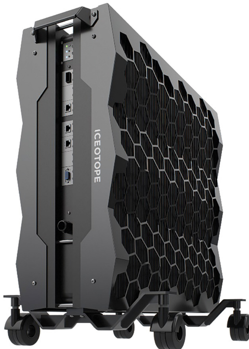
Figure 1. ICEOTOPE EdgeStation™ fan-free resilient workstation
