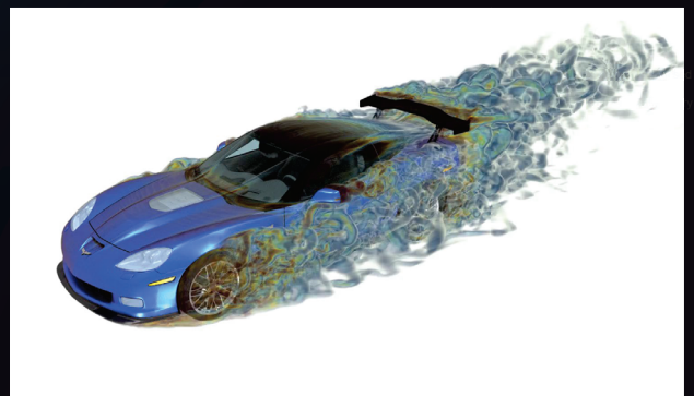
Corvette C6 ZR1 external aerodynamics 110M cells, SST-DDES, MRF for the wheels
